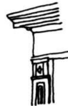
The intersection of Cornice, Fascia and Pilaster on a shop front without Console/Corbel bracket
